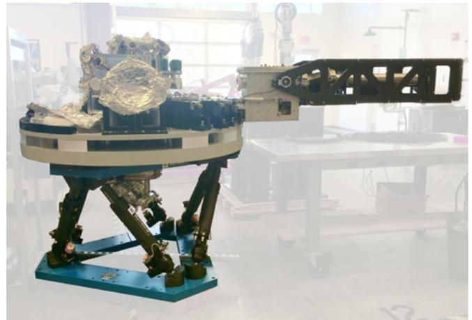
*JORAN actuators at LBL are longer to enable a  $\pm 12.5^\circ$  rotation around Z. This JORAN hexapod has also been customized to support a 3.2 tons payload.*
