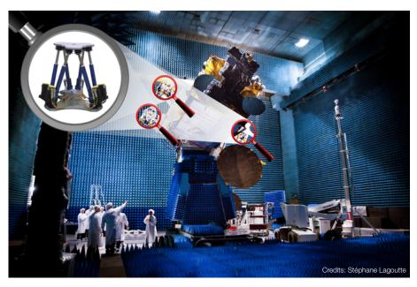
Four SIRIUS hexapods orientate the antennas of telecommunication satellite to test their performances before the launch. Thanks to the flexibility and pivot point configuration of these hexapods, this set up is adaptable to different satellite models.
