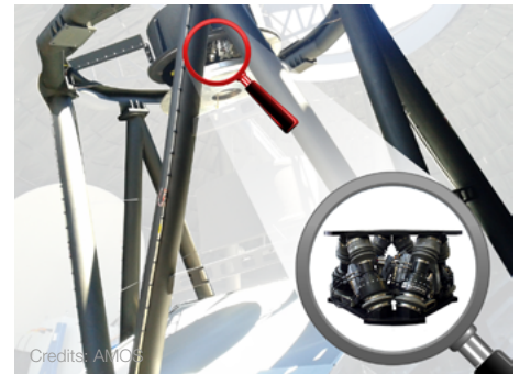
The hexapod is installed on Pan-STARRS-2 telescope at an altitude of 4267 m on Maui, Hawaii. A smaller version of SURES has been adapted as the secondary mirror is 600 mm diameter and weighs less than 110 kg.
